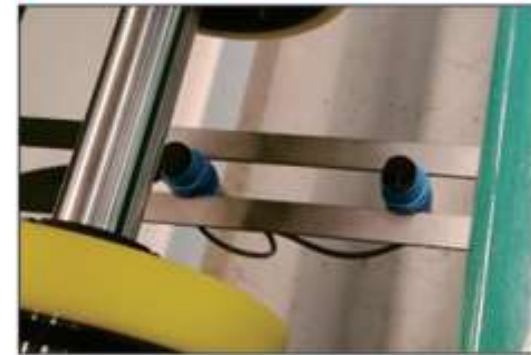
Detecting glass position on glass machinery
